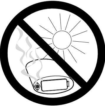
Use and store the metal detector only in normal temperature environments. Temperature extremes can shorten the life of electronic devices and distort or melt plastic parts.
